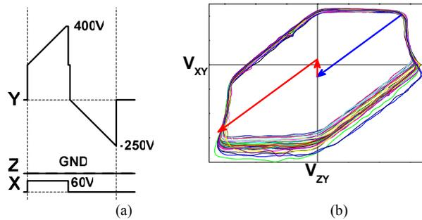
Fig. 11. (a) Improved reset waveforms suppressing unstable weak discharge and (b) Changes of cell voltage during reset period.
