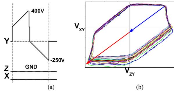
Fig. 10. (a) Proposed reset waveforms and (b) Changes of cell voltage during reset period.
