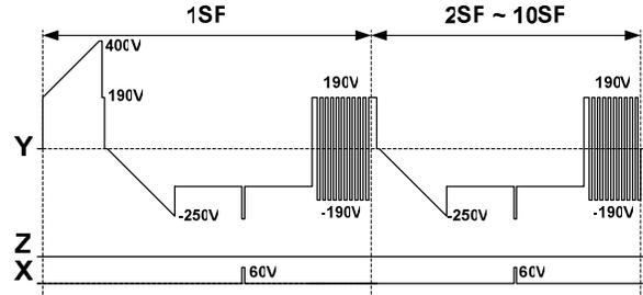
Fig. 6. Proposed driving waveforms applied to each electrode during 1 TV-field.
