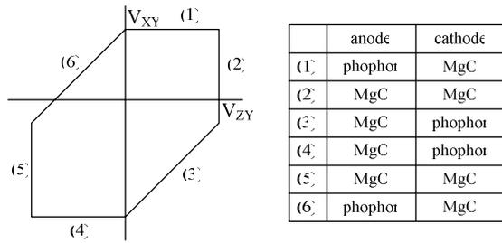
Fig. 7.  $V_t$  closed curve and surface layers covering electrodes which are participate in discharge corresponding to each side of  $V_t$  closed curve.
