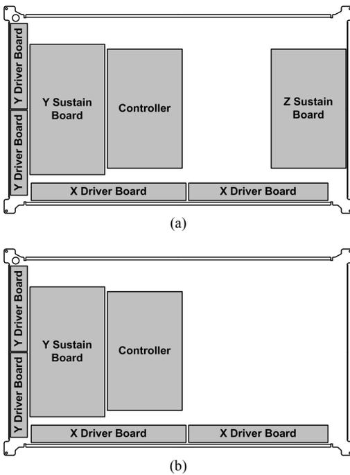
Fig. 13. Layout of driving circuit board for each driving waveform. (a) Conventional driving waveform, (b) Proposed driving waveform.
