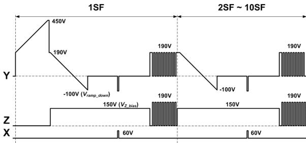
Fig. 3. Conventional driving waveforms applied to each electrode during 1 TV-field.
