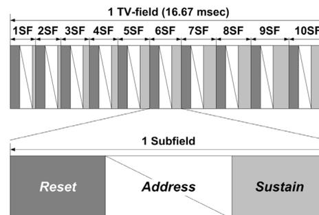
Fig. 2. Typical ADS (Address Display Separated) driving scheme.
