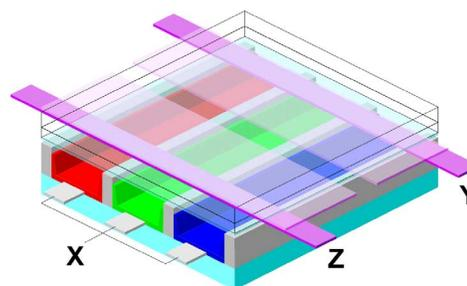
Fig. 1. Cell structure of typical three-electrode-type AC-PDP.
