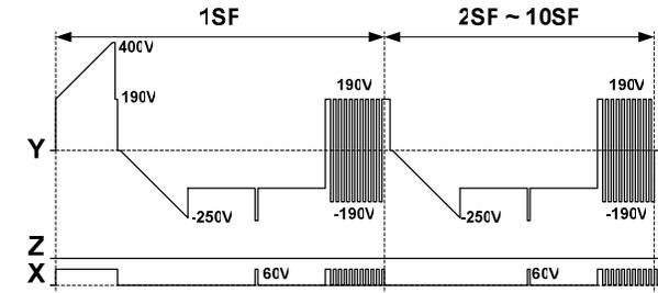
Fig. 12. Improved driving waveforms applied to each electrode during 1 TV-field.
