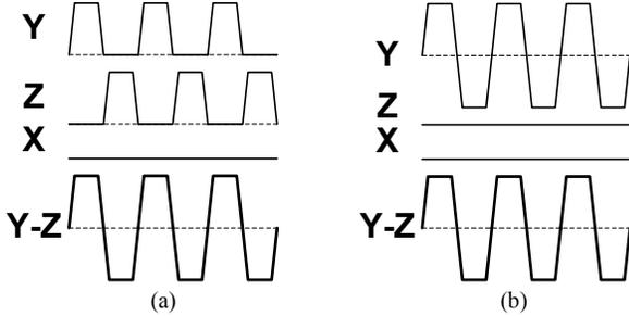
Fig. 4. Sustain waveforms. (a) Conventional driving waveform, (b) Proposed driving waveform.
