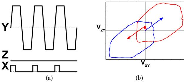
Fig. 9. (a) Improved sustain waveform suppressing phosphor degradation and (b) Movement of  $V_t$  closed curves during sustain period.
