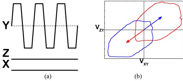
Fig. 8. (a) Proposed sustain waveforms and (b) Movement of  $V_t$  closed curves during sustain period.
