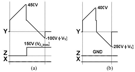
Fig. 5. Reset waveforms. (a) Conventional driving waveform, (b) Proposed driving waveform.
